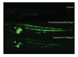
He said: "The zebrafish when modified with some clever genetics - it glows green in target tissues affected by chemicals - can be used as a highly sensitive tool to assess the interaction of environmental oestrogens in real time. It allows us to target our analyses of potentially damaging health effects more intelligently. And as it develops very quickly, we can investigate changes over a much shorter time period compared with the roach."
