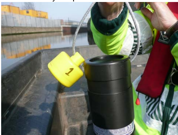
Receiver and temperature logger ready for deployment
