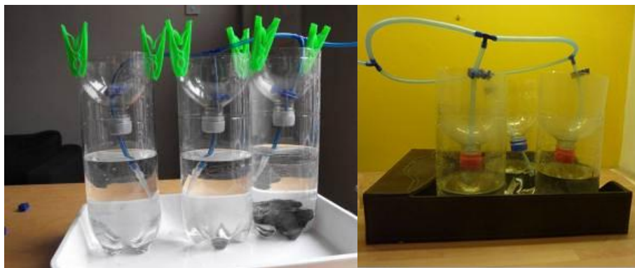
Final 3 vessel setup configurations; (inline) left, O-ring (right).
